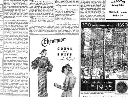
Bell System engineers long ago began to work out a way to clear city streets of overhead wires. The first telephone cables were crude affairs—a few wires drawn through a pipe. Continuous research brought forth improved designs, better manufacturing methods, cables of smaller size yet far greater capacity. The cable with the greatest number of wires today-3636-is 2%" in diameter.
