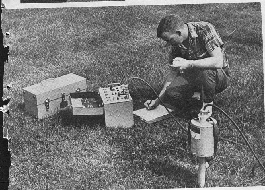
With the use of a newly developed instrument, the neutron meter, England measures soil moisture under a bluegrass cover. The meter, which utilizes radioactive material, simplifies soil moisture measurements. It is portable and, thus, can be used at other sites on this farm and on other Experiment Station farms to measure moisture at various depths in the soil profile.
