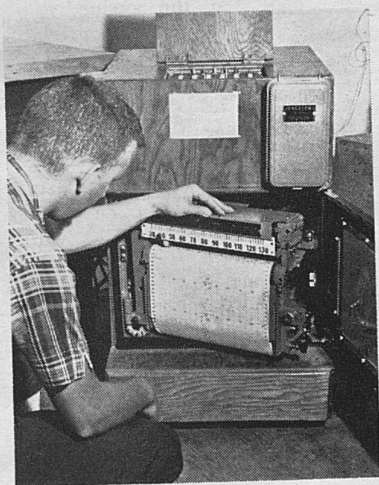
Graduate student Joe England inspects recorded data on the multilogger in the field laboratory. This instrument can record data from 144 separate temperature sites if desired. Thermocouples are used at the sites, with small wires connected to the multilogger.
