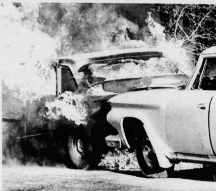
This is the result of a demonstration conducted to show what can happen to those who try to beat the current fuel shortage by carrying gas in the trunk of their car.
