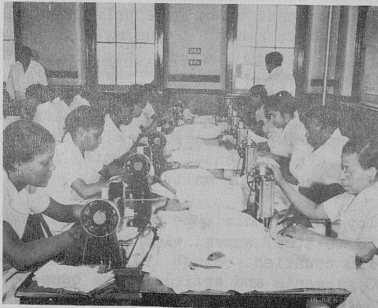
Team work method is used in WPA sewing room. Sewing machines are placed in lines to facilitate the flow of piece work.
