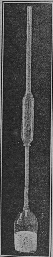
FIG. 12. — Proper method of running the milk into the test bottle.
