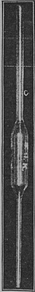
FIG. 3. — Standard milk pipette Babcock testing glassware and cream weights which have been thus examined and approved are permanently marked with the letters "S. G. K.," meaning "standard glassware, Kentucky."
