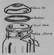
"Lightning" jar. Fit rubber in place on ledge at top of the jar. Put on glass lid, then push the long wire clamp tight over top of lid. Leave short wire loose. After the jars of food have been boiled and taken out of the boiling water . . . push this short wire down.
