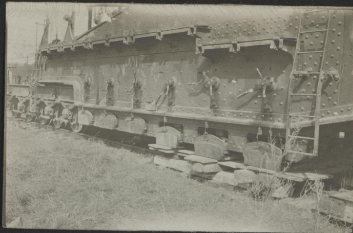
SHOWING HOW GUN CARRIAGE IS BLOCKED UP OFF THE WHEELS WHEN FIRING
