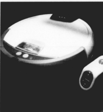
iRobot's Scuba uses a liquid solution to clean tile and vinyl flooring.
