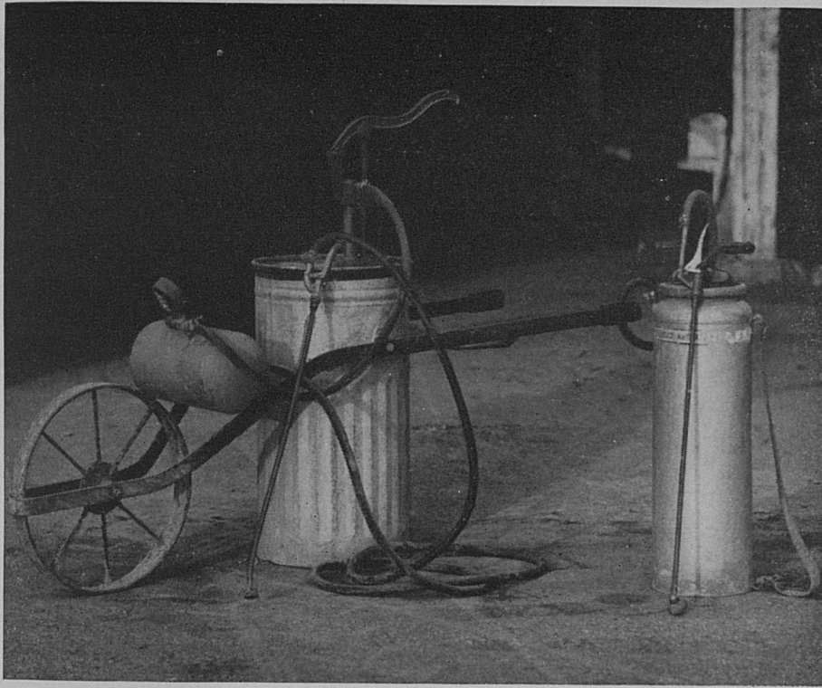
Fig. 2.— Both the wheelbarrow and the knapsack type of sprayer are generally satisfactory, but for the larger gardens the wheelbarrow type is more practical.
