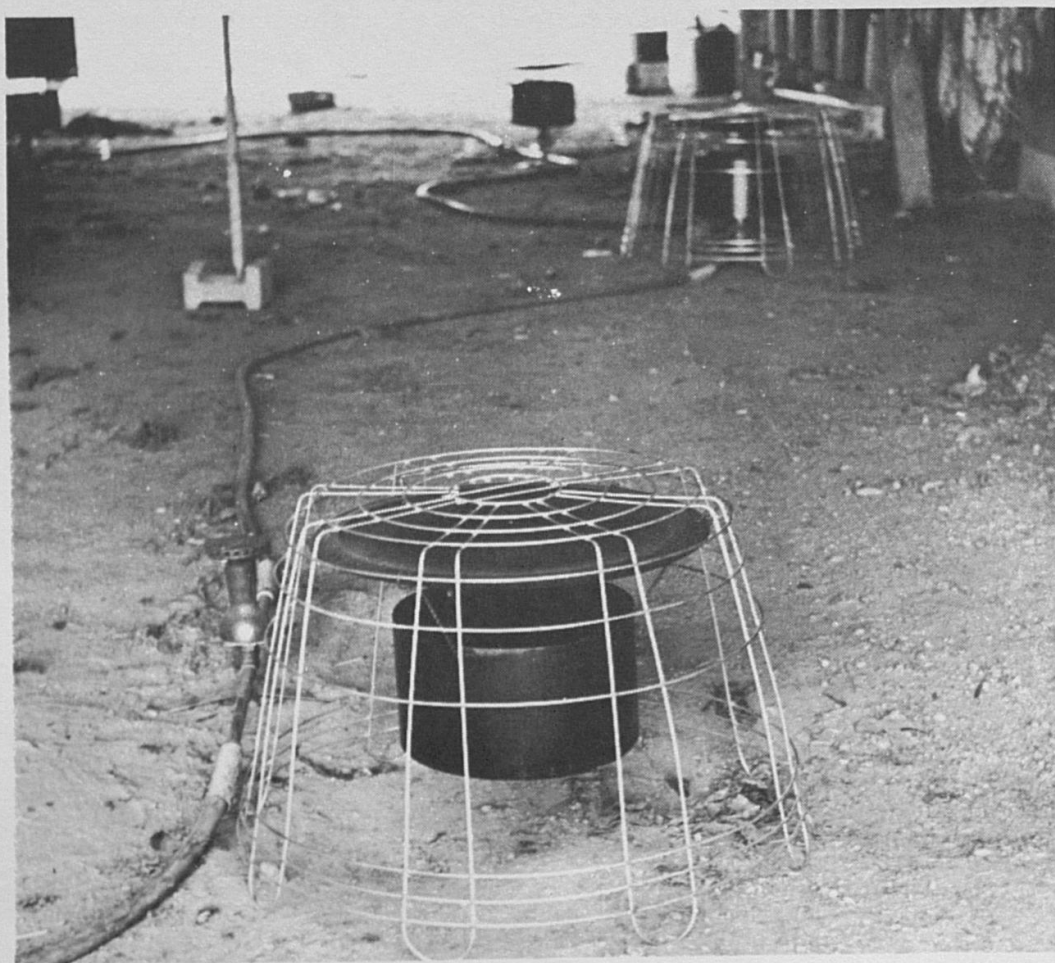
Fig. 31.—This small gas unit has a maximum heat output of 30,000 B.t.u. per hour.
