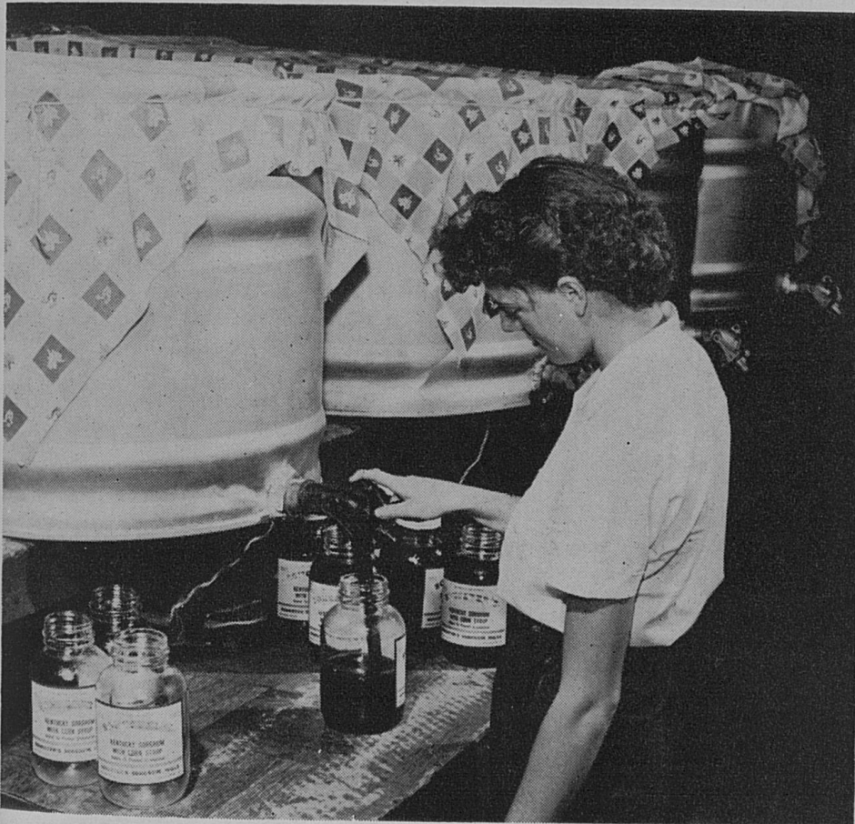
Fig. 7.— The syrup is dispensed into glass containers through a molasses spigot. The muslin-covered dispensing tanks insure cleanliness until the syrup is bottled.
