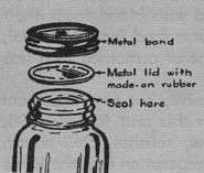
**2-piece cap.** Place metal lid, with rubber side down, on top of jar. Screw band on firmly, and **do not tighten** it again even after the jar of food is taken from the boiling water.
