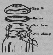
"Lightning" jar. Fit rubber in place on ledge at top of the jar. Put on glass lid, then push the long wire clamp tight over top of lid. Leave short wire loose. After the jars of food have been boiled and taken out of the boiling water . . . push this short wire down.
