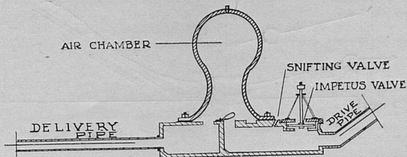
Diagrammatic section of a hydraulic ram.
