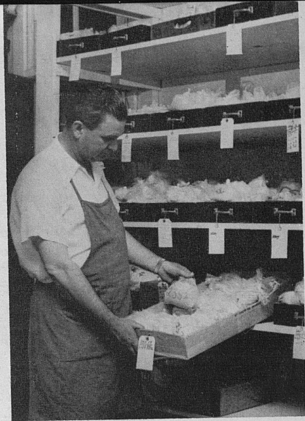
(right) Reserve portions of feed samples are stored in plastic bags for additional rechecking if requested. Samples are normally kept on file for 3 months.
