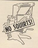
A common cause of machine squirts lies in faulty metal pot temperature control.
