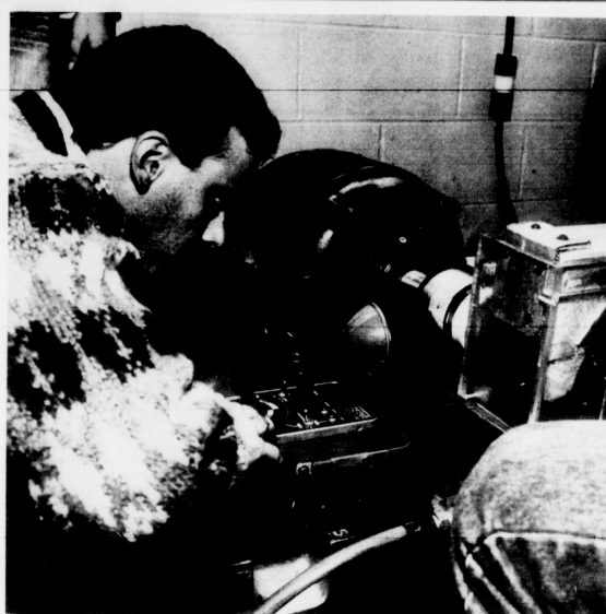
REVVED UP: Chris Budniak, a mechanical engineering junior, measures the revolutions per minute of an electric motor using a stroboscopic camera. Photo by RANDAL WILLIAMSON/Kentucky Kernel Staff
