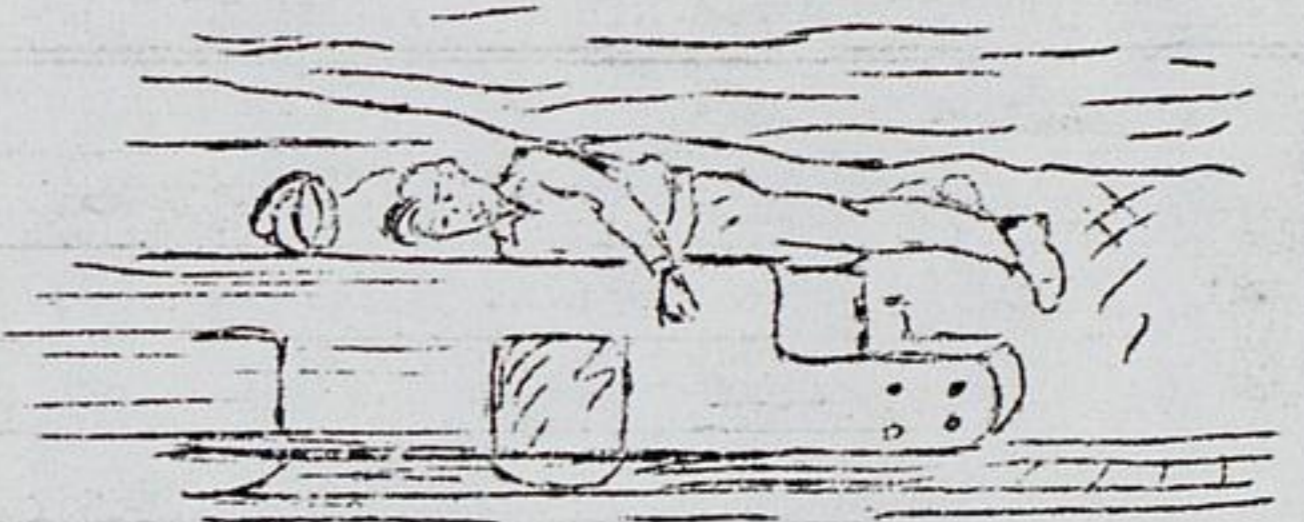
DRAGGED OVER TOP OF MOTOR, IN LOW TOP, BY REEL CABLE.
