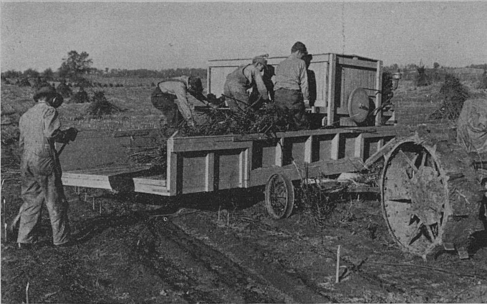
Machine for beating out hemp seed. This home-made machine was designed by the Agricultural Engineering Division. Over twenty of these machines were built and used in Kentucky this year. They saved much labor.
