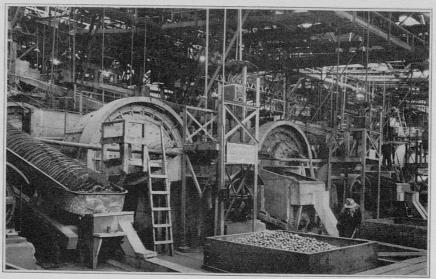
FIGURE 41.— MODERN CONCENTRATION METHODS REQUIRE THAT ORE BE CRUSHED AND GROUND UNTIL THE LARGEST PARTICLES RESEMBLE FINE SAND.
