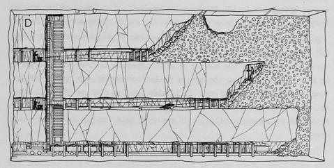
SUBLEVEL INCLINED CUT-AND-FILL STOPING RETREATING SYSTEM
