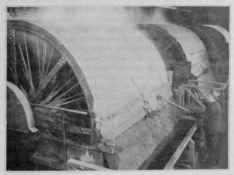
FIGURE 44.- CONCENTRATES MUST BE DEHYDRATED
