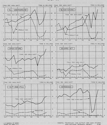
Figure 23.- PRODUCTION OF COPPER AND OUTPUT PER WORKER AT UNDERGROUND COPPER MINES, BY MINING METHOD, 1917-36
