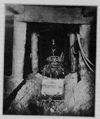
FIGURE 37.- A SCRAPER LOADER IN A WESTERN COPPER MINE
