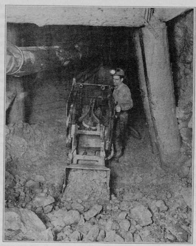
FIGURE 36.- THE USE OF MECHANICAL LOADING MACHINES
