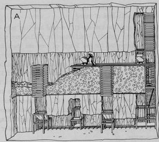
HORIZONTAL CUT-AND-FILL STOPING DISTRIBUTION OF WASTE FILLING BY HAND TRAMMING
