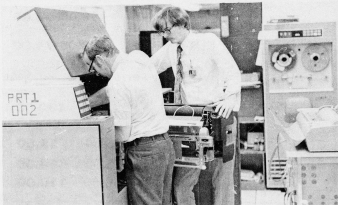
Two IBM repairmen replace broken components in a printer at the UK Computer Center. (Kernel photo by Chuck Combes).
